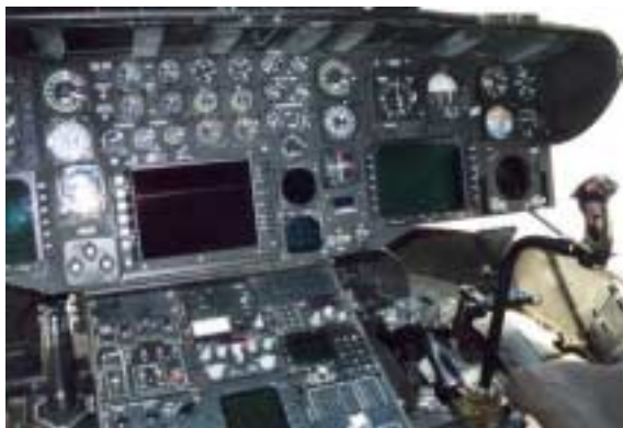
Figure 9. MH-53 PAVE LOW III Cockpit (Sidearm Controller at Lower Left)
