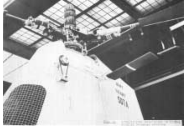
Figure 3. Longitudinal Stabilizer Installed on the Piasecki XHJP-1, from [6]. Airfoil Pitch Change Actuation Mechanism Controls Trim Speed.
