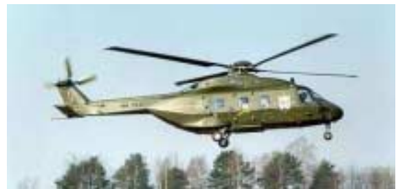
Figure 28. The NH-90 Recently Began Flying Under Fly-by-Wire Flight Controls Without Mechanical Backup.
