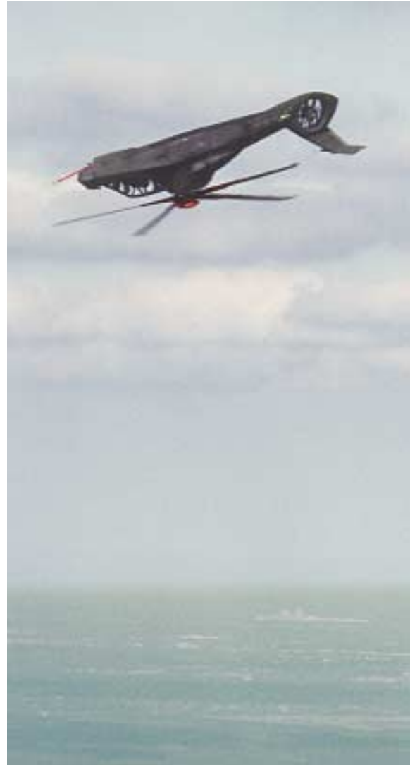
Figure 26. RAH-66 Comanche Demonstrating Full-Envelope Capability with a Split-S Maneuver.
