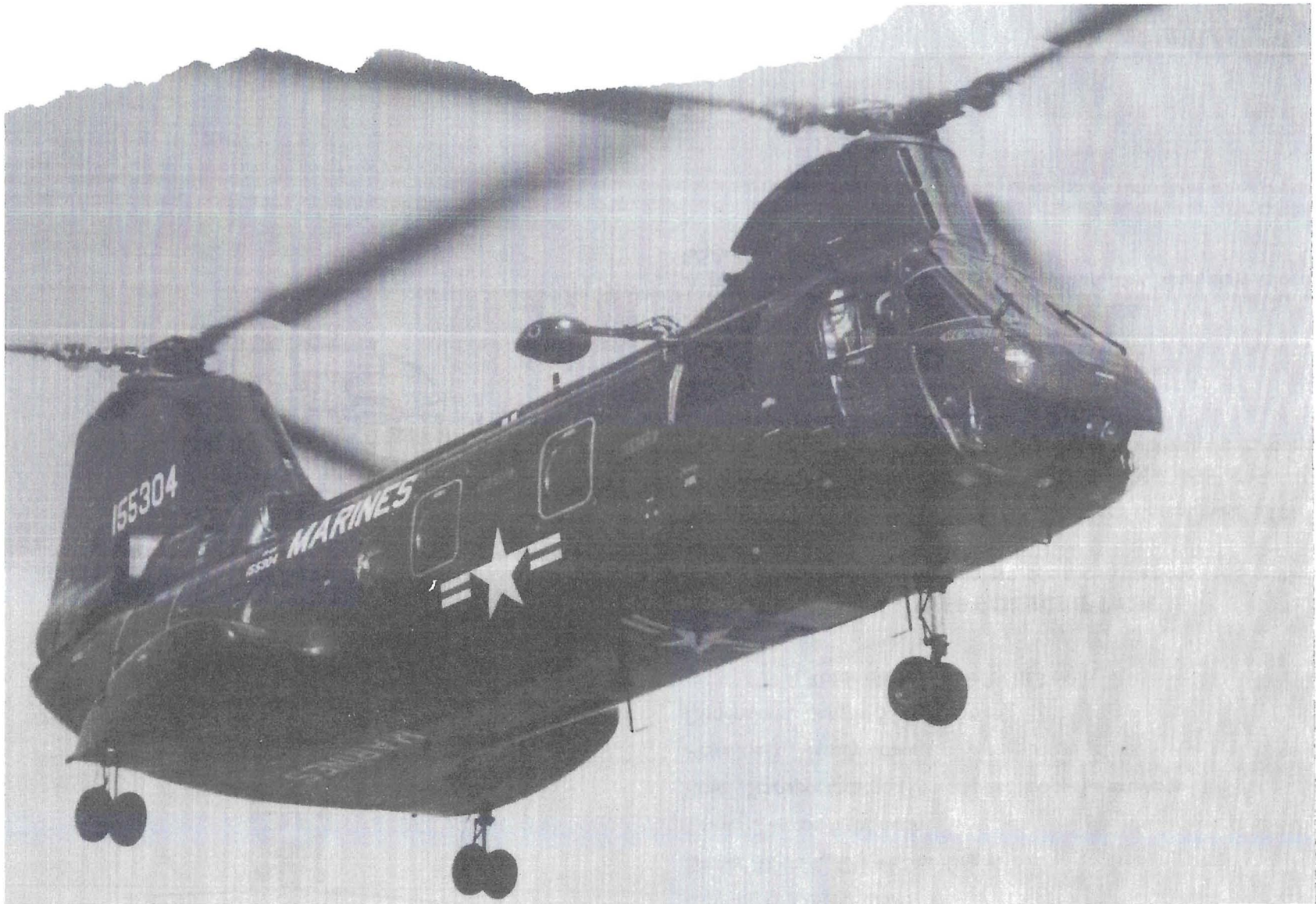
The Sea Knight is a land- and ship-based aircraft. There are many versions. When comparing this aircraft and the CH-47 Chinook, note the differences in the landing gear, engine mounting, fuel pod size, and size of the aircraft.
