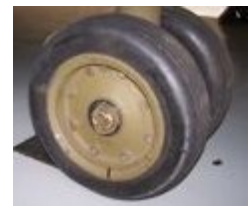
Early CH-47A Aft Landing Gear (hard rubber)
