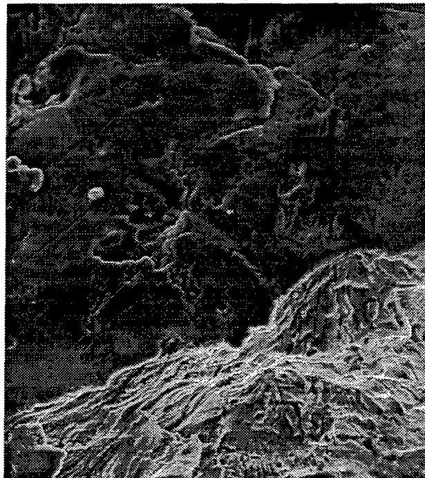
Figure 20. Magnified SEM of Figure 19, Showing Intergranular Attack on the Surface of the Bore Adjacent to the Primary Fracture Origin; Magnification 200x.
