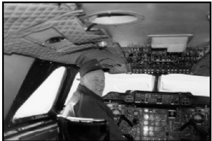
While on board the Concorde , I got an opportunity to check out the cockpit. For such a speed demon, it has an old-fashioned steam gauge instrument panel. The plane is single-aisle, with two seats each side. It can carry 100 passengers, who pay $7,500 for a New York-Paris round trip. The airplane carries 25,000 gallons of fuel for a one-way trip. □ 5
